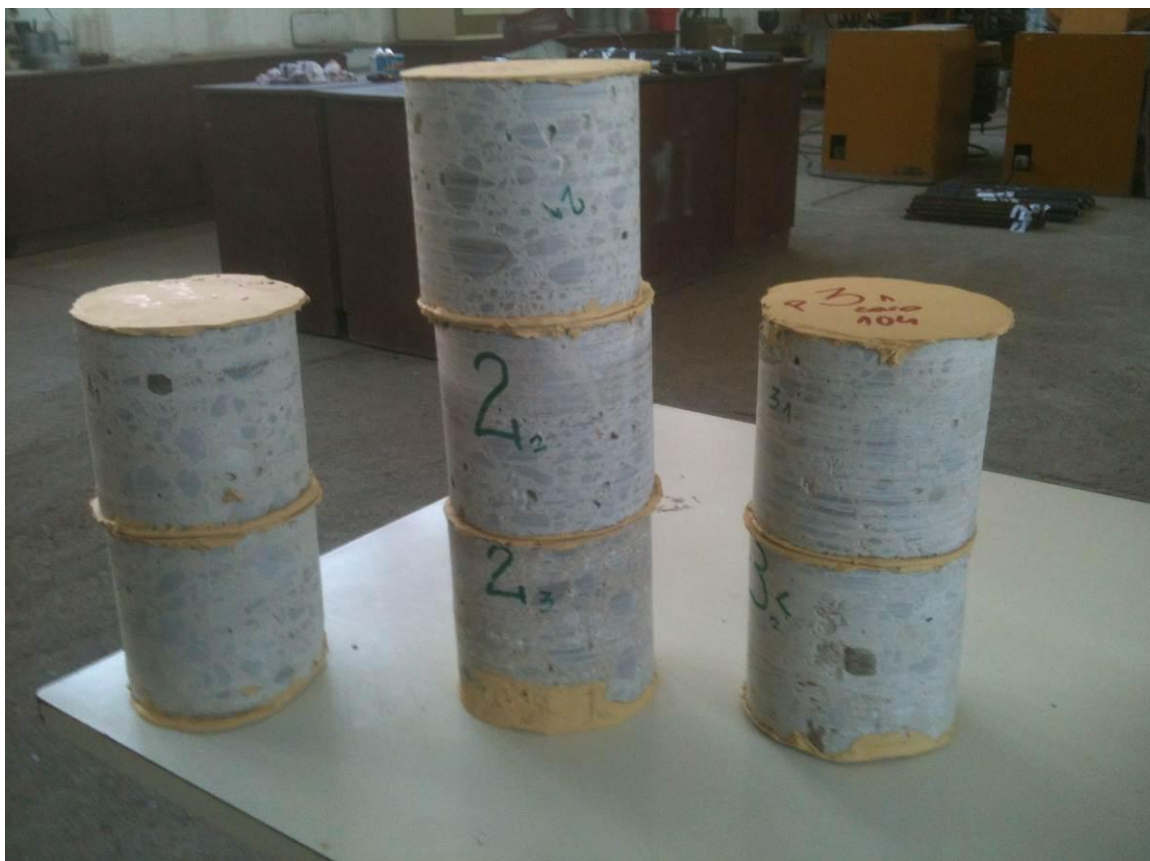
Picture 1. Samples from RC slabs of Pier 1 prepared for testing
