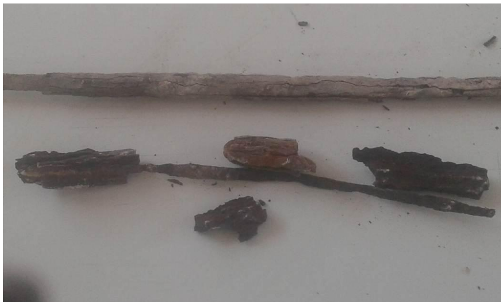
Picture 3.b) pieces of cracked stirrups from transverse girder
