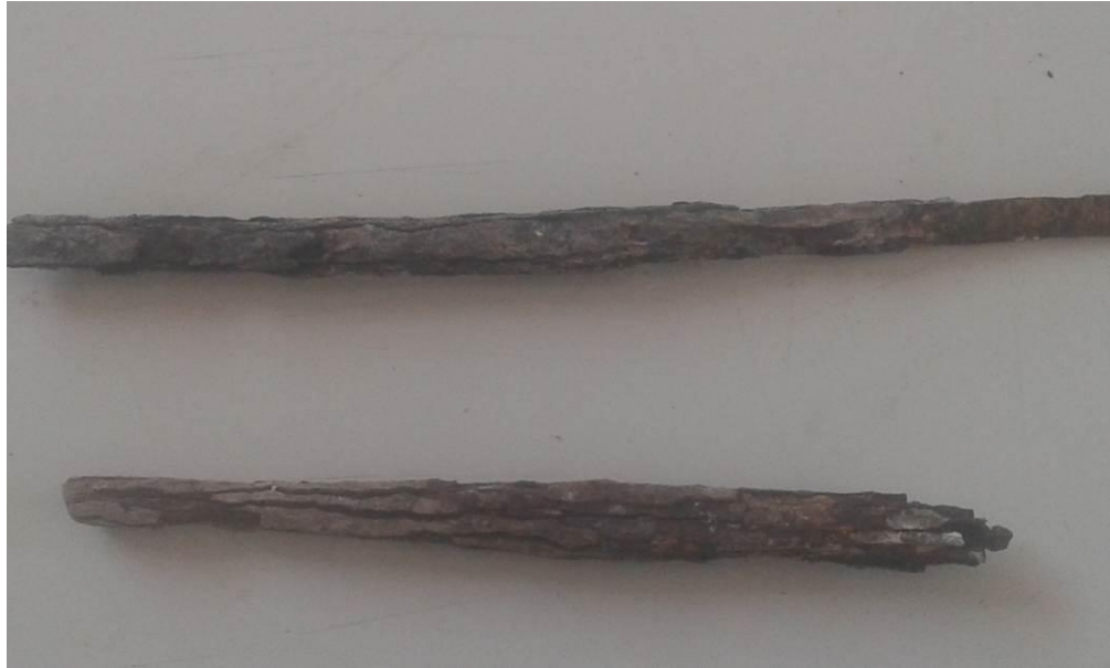
Picture 3.a) pieces of cracked stirrups from transverse girder
