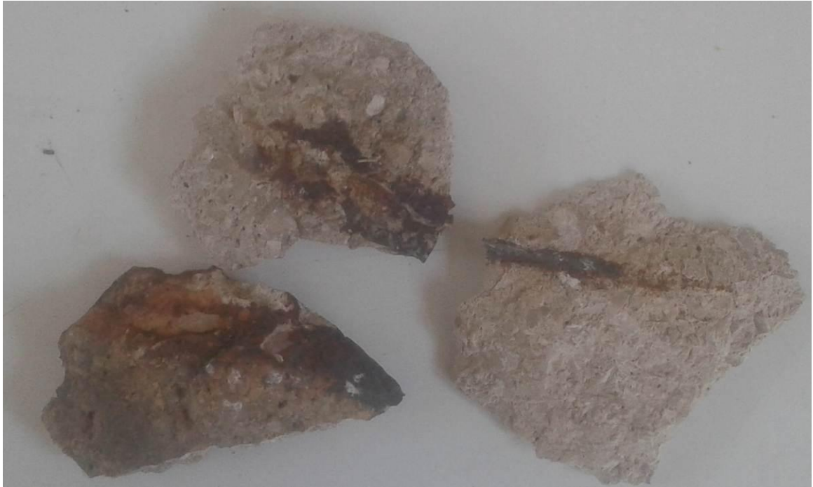
Picture 4. pieces of fallen-off concrete with traces of reinforcement corrosion
